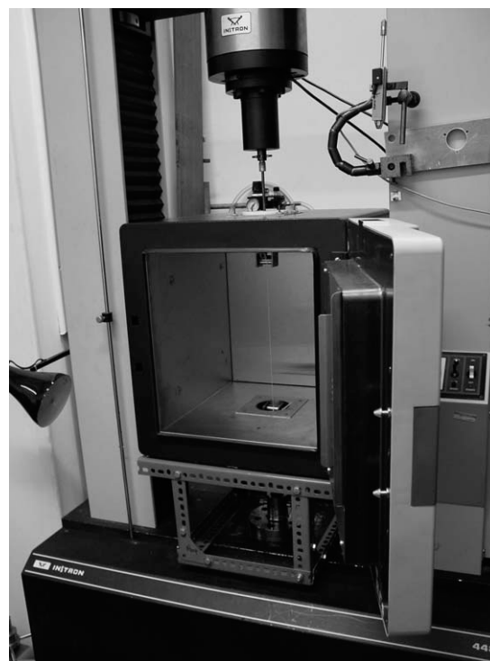
Figure 6 Experimental set-up for tensile and SIM tests.
